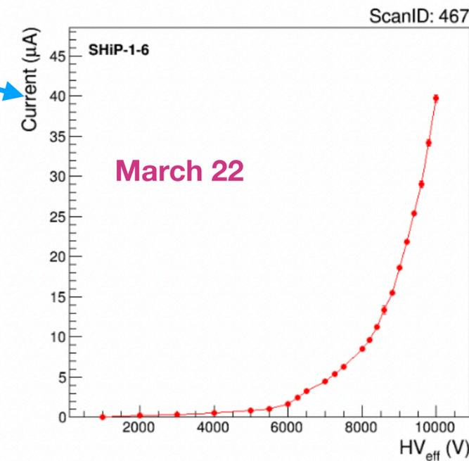
HV scan of Ship chamber
