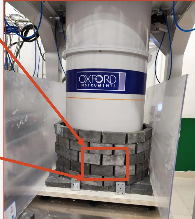
Stacked configuration with the **250 Kg lead castle shielding**
