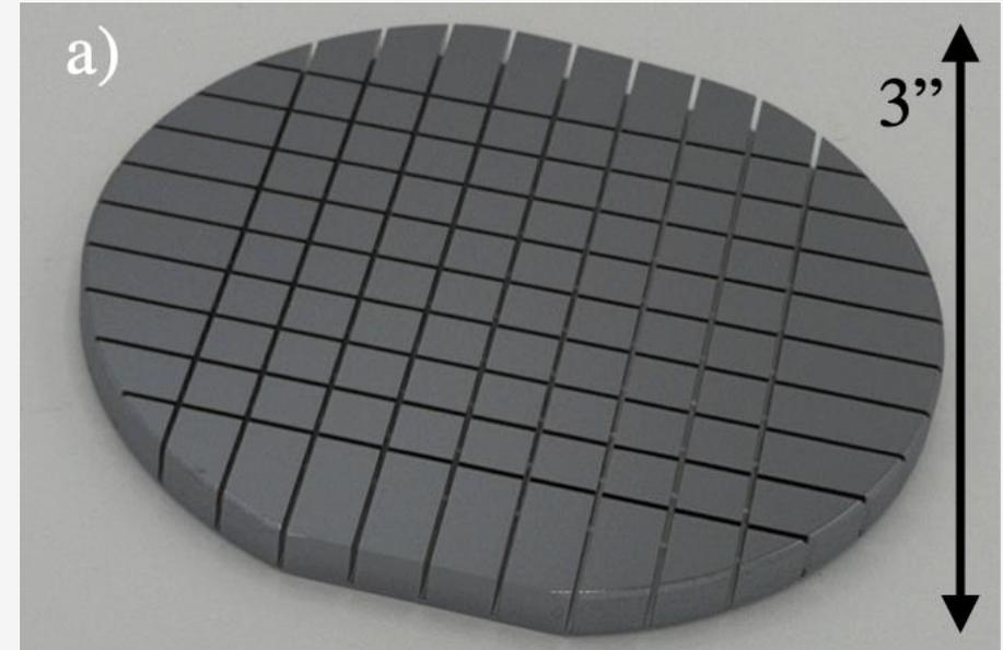
KID array on the other side of the wafer hosting 60 resonators (60 nm Al)
