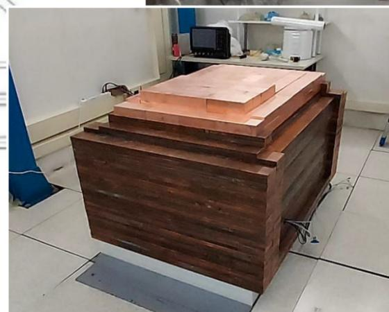
Shielding for crystal testing
