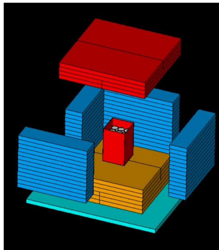
3x3 NaI matrix with 15 cm copper shielding + 40 (60) cm polyethylene lateral and top (bottom)
