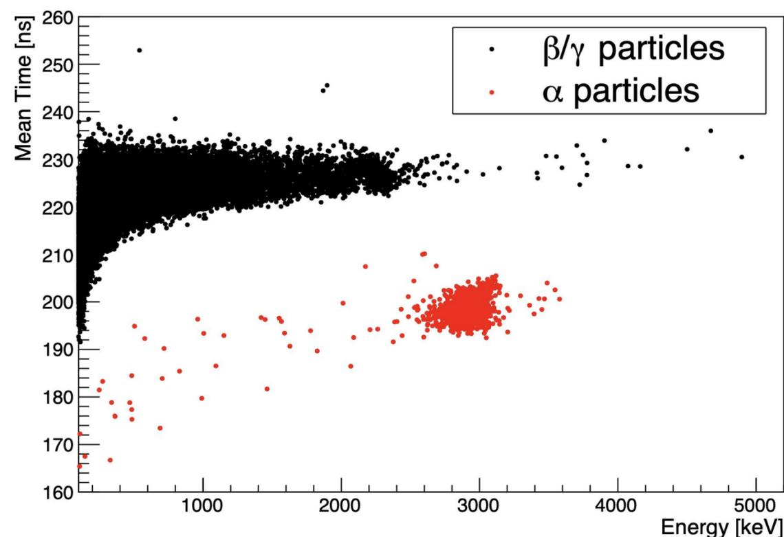
Mean time against energy to identify the  $^{210}\text{Po}$  background as a proxy of  $^{210}\text{Pb}$
