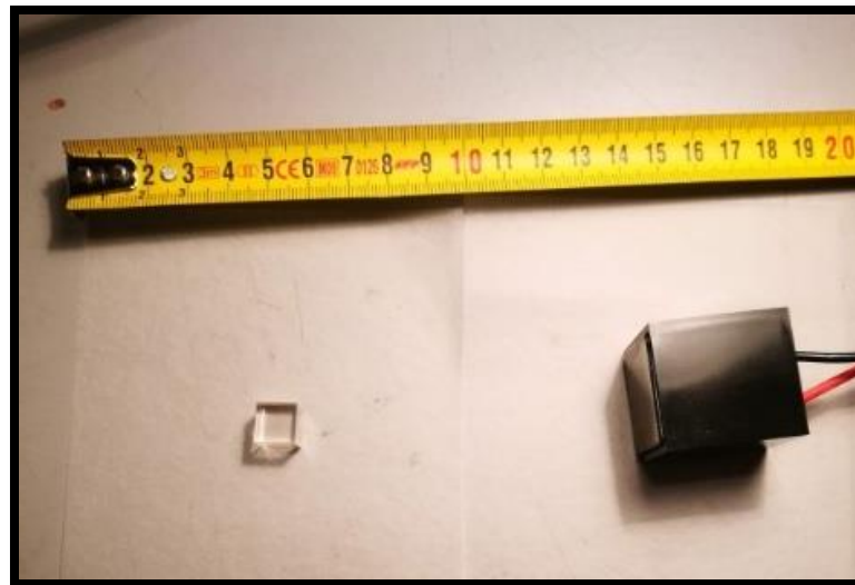
\text{ZnWO}_4 crystal = 10 \times 10 \times 10 \text{ mm}^3 (detector of reduced dimensions to investigate neutron single-scattering)
