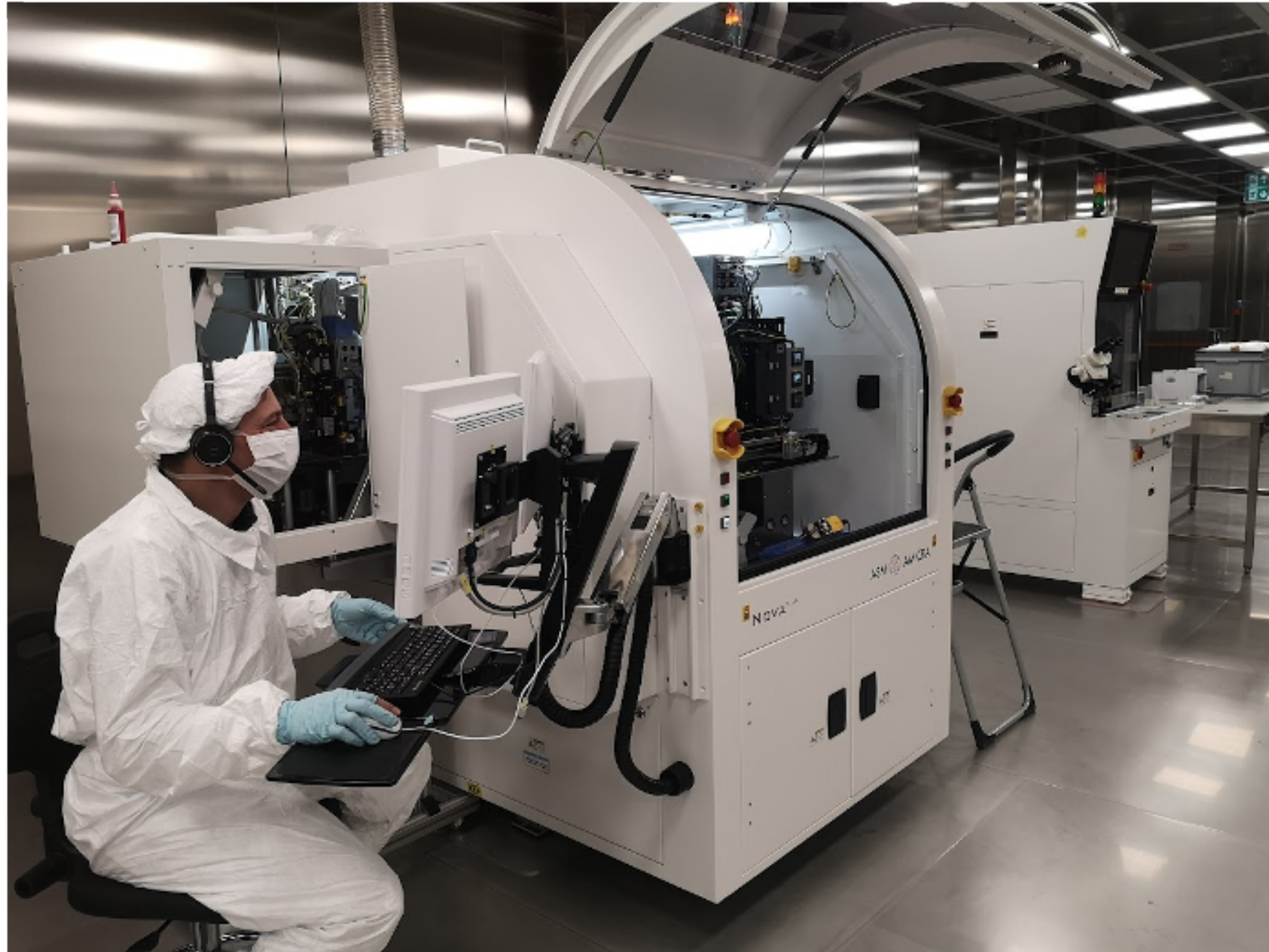
Flip Chip Bonder (Amicra) Tiles of 24 SiPMs are assembled
