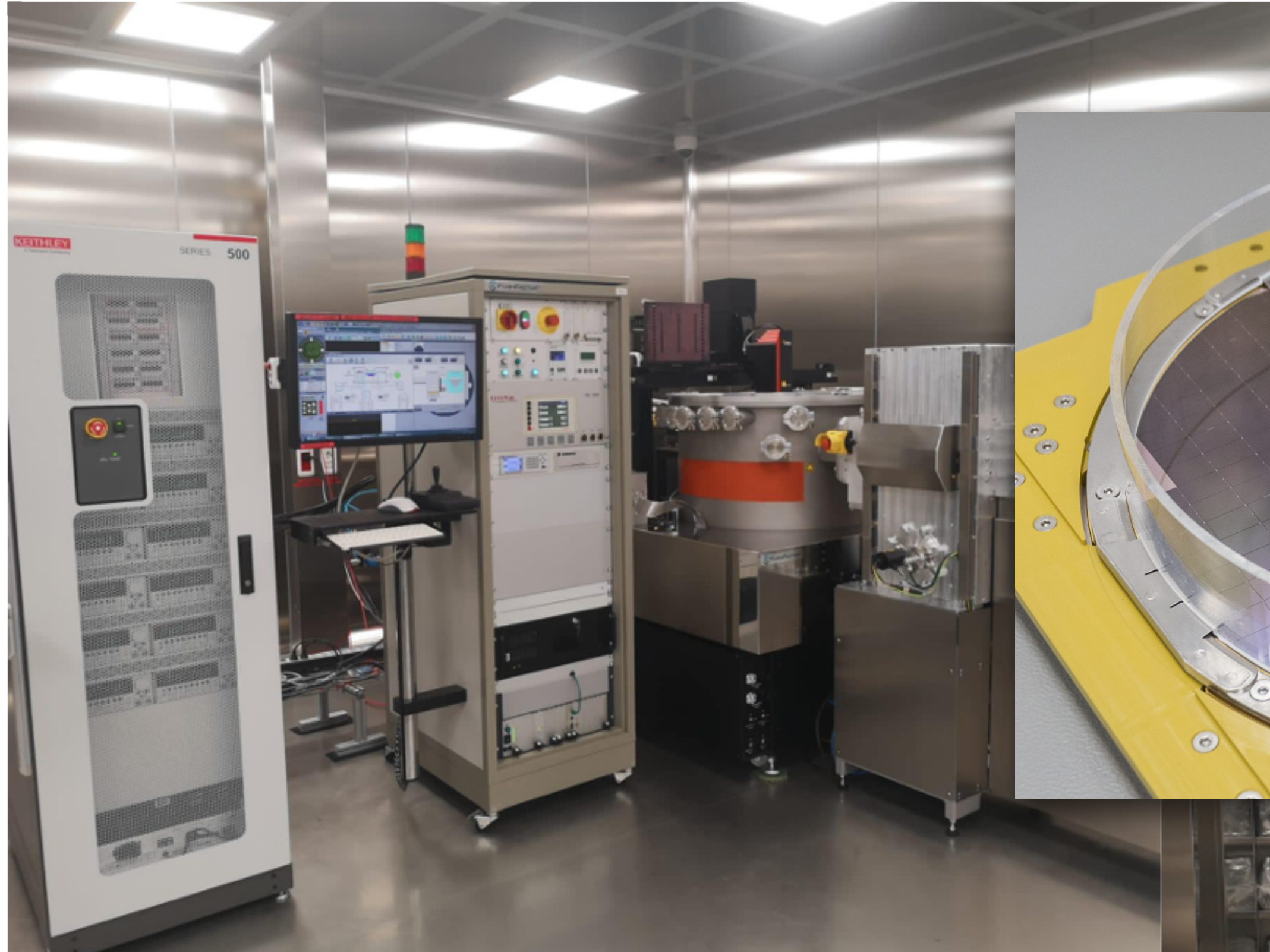
CryoProbe (FormFactor) test single SiPMs in wafer
