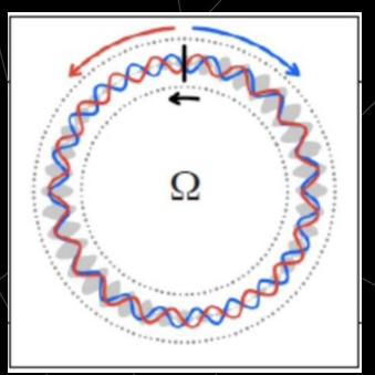
two counterpropagating beams in a closed path (interferometer with equal arms)
