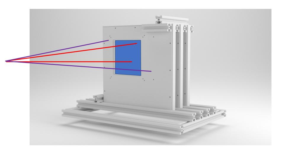
It can be very important that all the tracks pointing to TW are those which cross the active area of MSD, to minimize problems of interactions in passive materials
