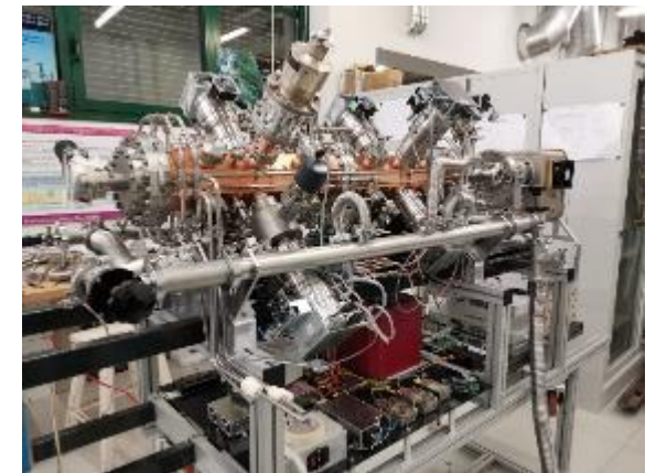
Portable PIXE system based on an RFQ linac built by CERN and LABEC
