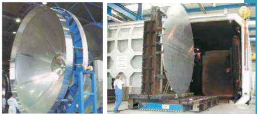
Fig. 4.7: An impressive example of an EB-welding application. In a huge vacuum chamber two 70-mm-thick aluminium plates, with a diameter of 6 metres, are joined with a 'single-shot'. It is the basic material used in forging and machining the main stage of Ariane-rocket tanks.
