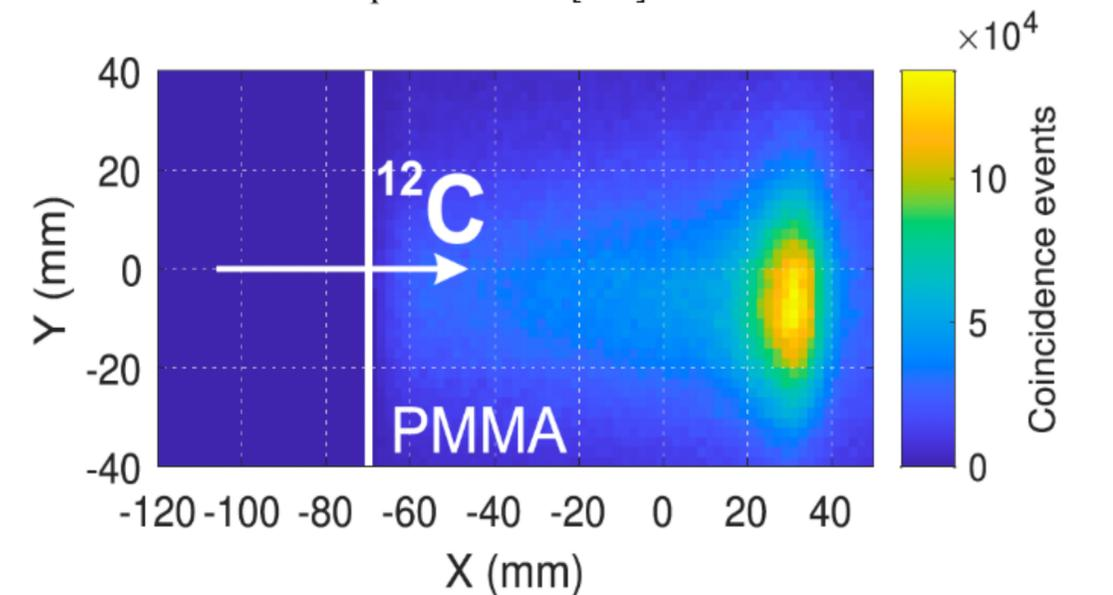
PET range uncertainty after delivering  $1.6 \times 10^7$  ions in 4 spills (19.2 s total): **0.04 mm**, **0.7mm**, and 1.3 mm for  $^{10}\text{C}$ ,  $^{11}\text{C}$ , and  $^{12}\text{C}$
