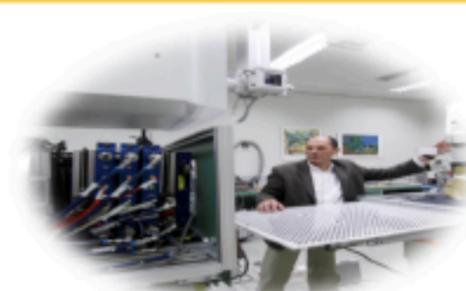
Visualize RIB using BASTEI PET camera and hybrid  $\gamma$ -PET detector
