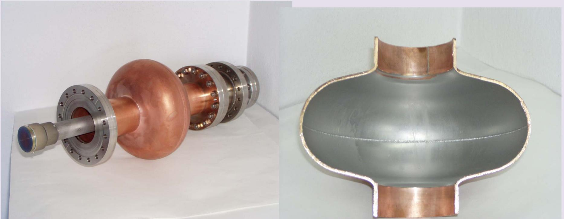
**The coated single-cell has been cut along its symmetry axis in order to perform an analysis of the inner surfaces.**
