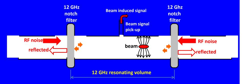
RF noise has to be filtered at both the pick-up sides.
