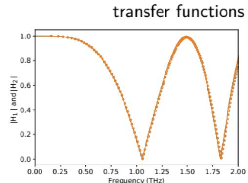
Transfer functions  $H_{1,2}$  for the "classical" crystal & waveplates orientations
