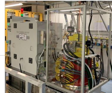
All waveguide RF components including the XBOC and phase shifters were designed and built at PSI, Klystron: CPI VKK-8311 **50 MW X-band**
