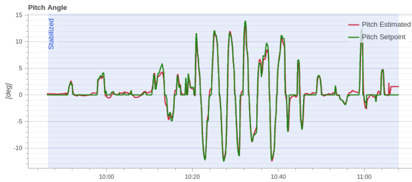
Figure 8: Pitch angle tracking with implemented attitude controller.
