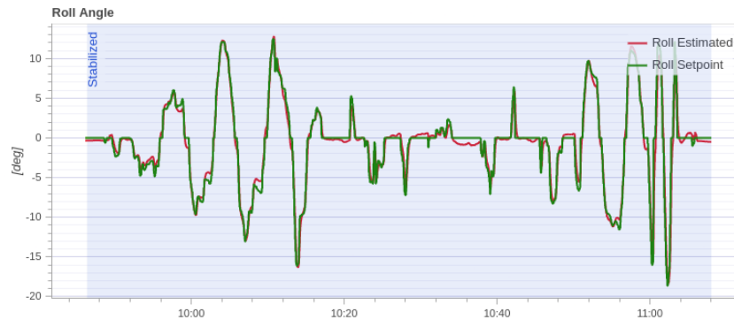
Figure 7: Roll angle tracking with implemented attitude controller.
