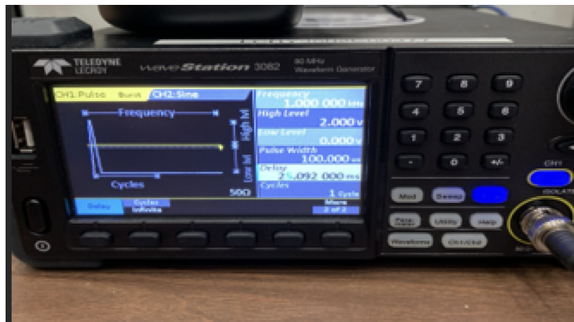
Figure 13: Picture of the pulse generator with, as example, the settings to acquire the first kick of the train of 8.
