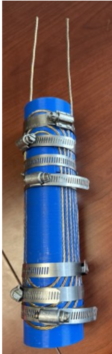
Figure A.2: The final magnet
