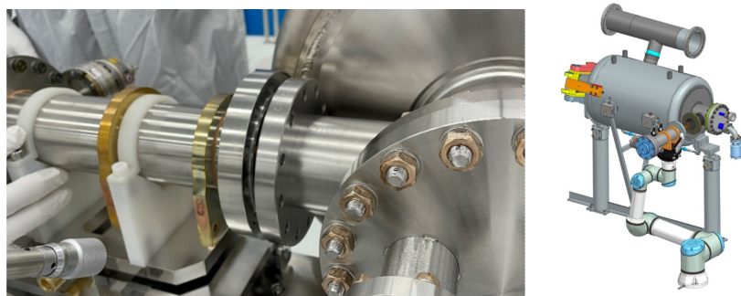
Figure 1.8: Manual and robotic flange alignment for a power coupler insertion
