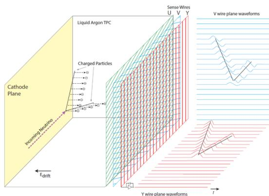
Fig. 3: An illustration of a neutrino-Argon interaction inside of a LAr-TPC.  $\text{Ar}^+$  ions drift towards the cathode on the left and  $e^-$  drift towards the anode on the right. Signals get registered for every wire.
