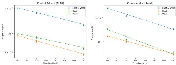
Fig. 13: Log scale plots showing trigger rate in function of threshold, for NuMI-like gates, in the central-corner adder setups. A linear fit has been shown to verify that this trend match with the exponential model.
