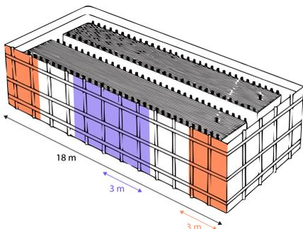
Fig. 10: Details of a cryostat module, revealing its segmentation into three 6-meter-long windows, each hosting 30 PMTs on both the west and east sides. In the above illustration, red denotes the corner adder boards, whereas blue indicates the central adder boards (each board processes the signal of 15 PMTs).
