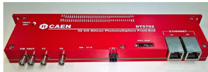
Top: Scheme of the ICARUS TPCs and CRT system modules. Bottom: The FEB in its case.
