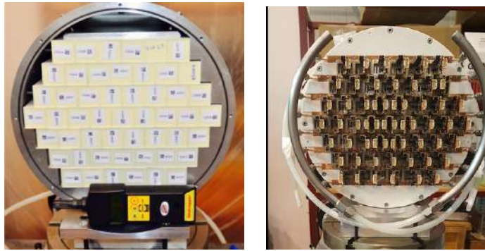
Figure 6.1: Pictures of the Module-0 during assembly: frontal view with crystals (Left) and back view with SiPM and FEE chips (Right).
