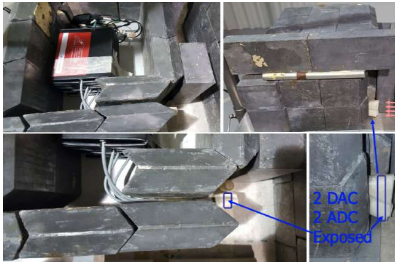
Figure 5.19: Experimental setup prepared for the irradiation of the ADC and DAC components.
