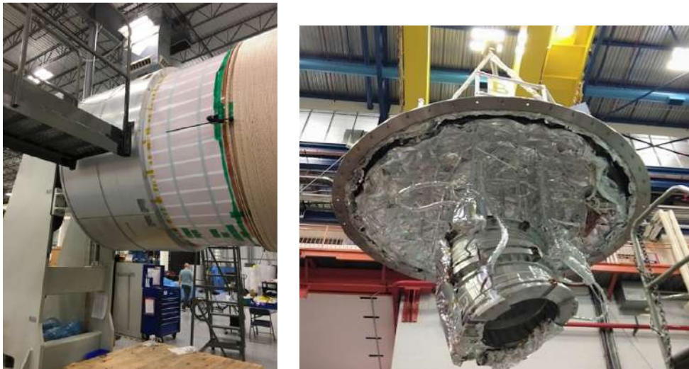
Figure 2.15: Left: picture of the winding procedure of the PS. Right: TS unit, attached to the top of the cryostat, being craned to the cryostat for cold testing.
