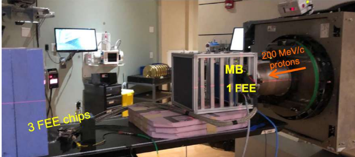
Figure 5.21: Experimental setup used for the SEU test of the calorimeter FEE chips.
