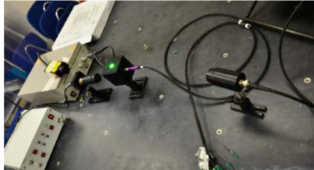
Figure 4.22: Picture of the light distribution system prototype tested at INFN-LNF, with a green laser and an integrating sphere.
