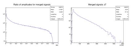
These are the projections for the ratio  $\frac{B}{A}$  and for the  $\Delta t$  of the merged signals:
