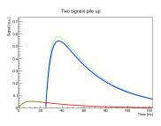
**Current model:** event signal at  $t = 25 \, ns$  merged with the background one at  $t = 0 \, ns$ .
