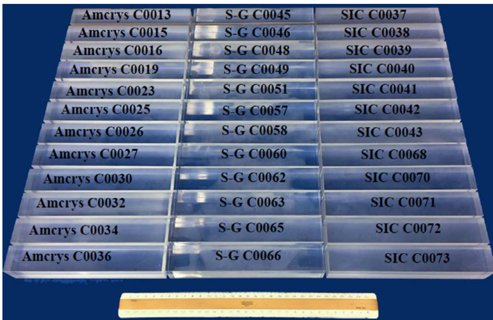
Figure 4.1: Picture of the pre-production crystals received from Amcrys, Saint Gobain and Siccas vendors.
