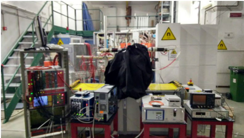
Figure 6.6: Test Beam experimental setup inside the BTF hall. The Module-0 is covered by a black blanket.
