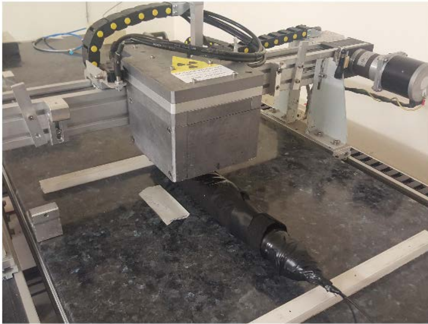
Figure 4.17: Experimental apparatus for RIN measurements: a motorized cart transport a strong ^{137}\text{Cs} source over the CUT.
