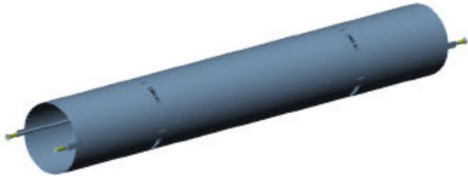
Figure 6.3 – 70 K Thermal Shield Assembly. (T. H. Nicol et al.)
