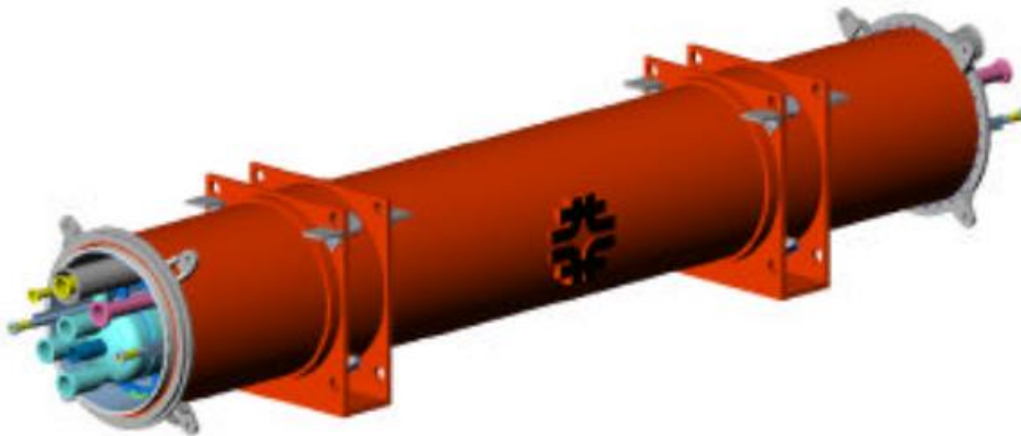
Figure 6.6 – Complete Magnet Assembly. (T. H. Nicol et al.)
