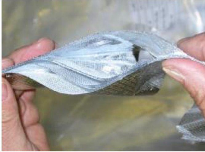
Figure 7.6 - MLI stack in a blanket. (V. Parma et al.)
