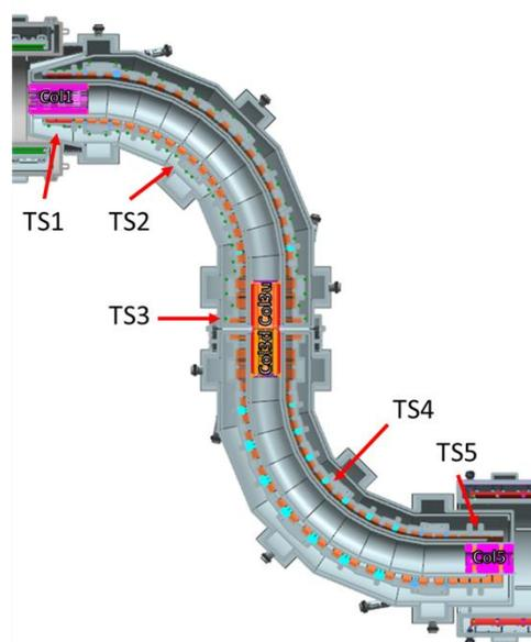
*Figure 3.1 - The Transport Solenoid with the significant components identified.*
