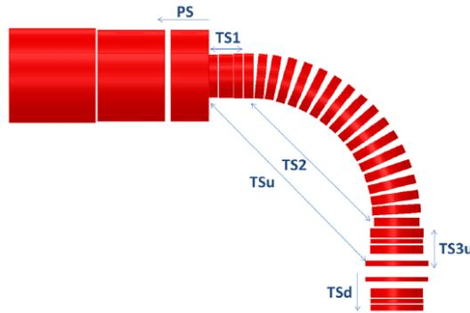
*Figure 3.4 - TSu coil locations with respect to the adjacent magnets.*
