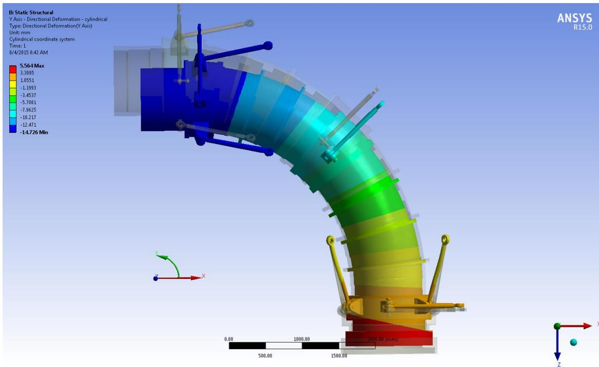
Figure 3.8 –Tsu support lug displacement during cool-down (Y axis).
