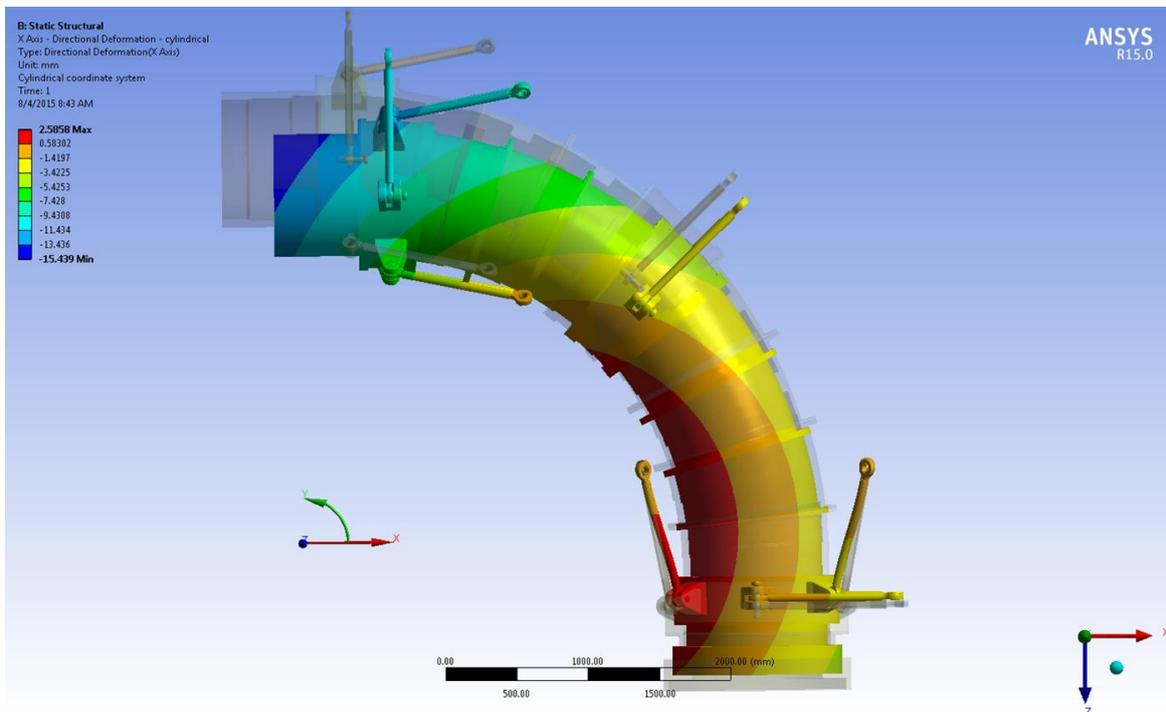
Figure 3.9 –Tsu support lug displacement during cool-down (X axis).
