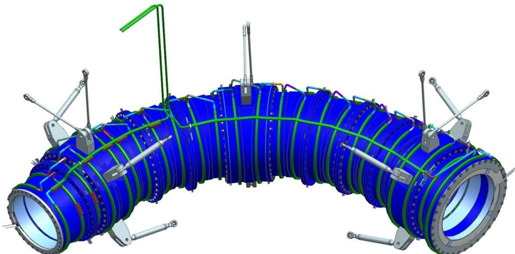
*Figure 3.7 – TSu cold mass assembly.*
