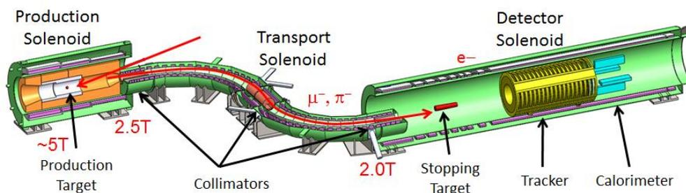
*Figure 2.1 – The Mu2e experiment overview*
