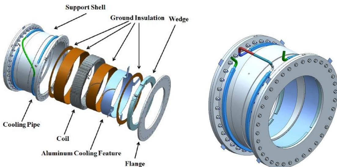
*Figure 3.6 - A typical TS coil module.*
