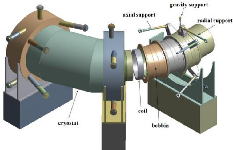
*Figure 3.5 - TSu components (partial cutaway).*
