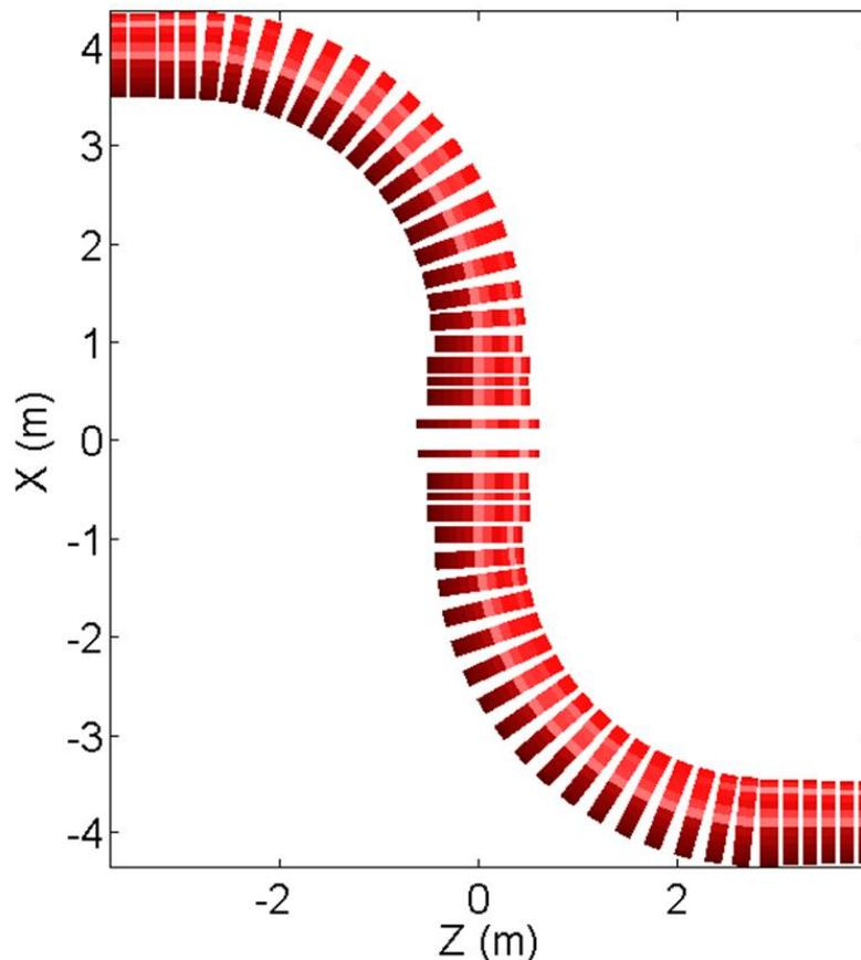
Figure 3.2 - Design of the Transport Solenoid.
