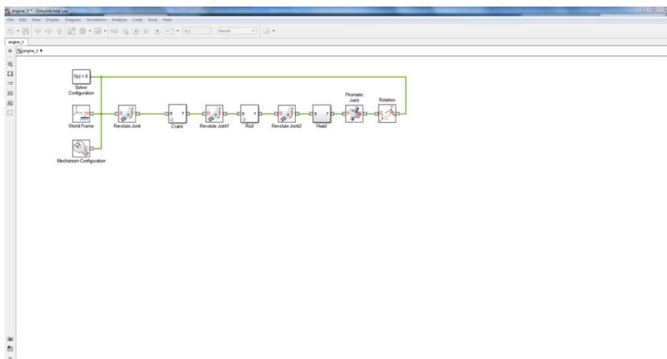
Figure 4.1 – Example of the structure of a mechanical model, made through SimMechanics.
