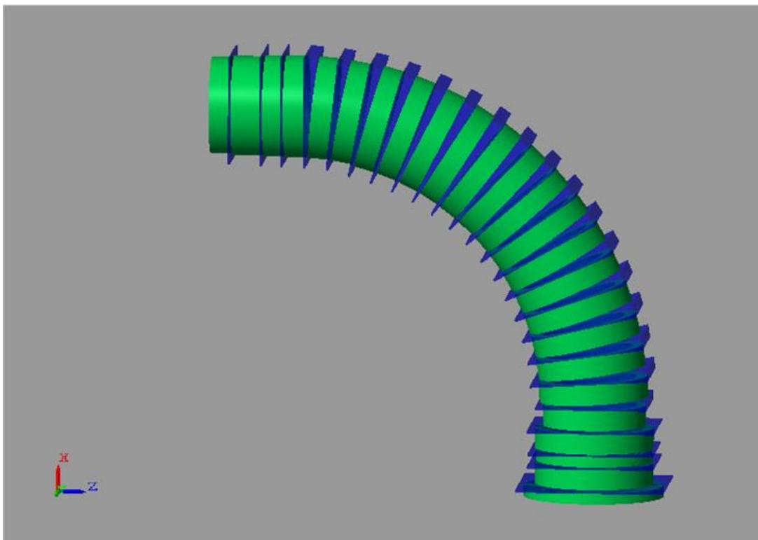
*Figure 4.6 – The TSu mechanical model, made through SimMechanics.*
