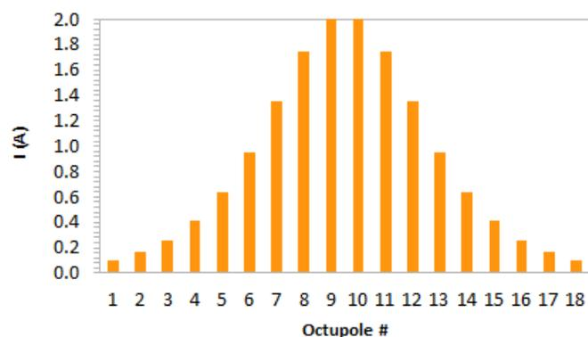
Figure 1 Currents for magnets in the tunnel
