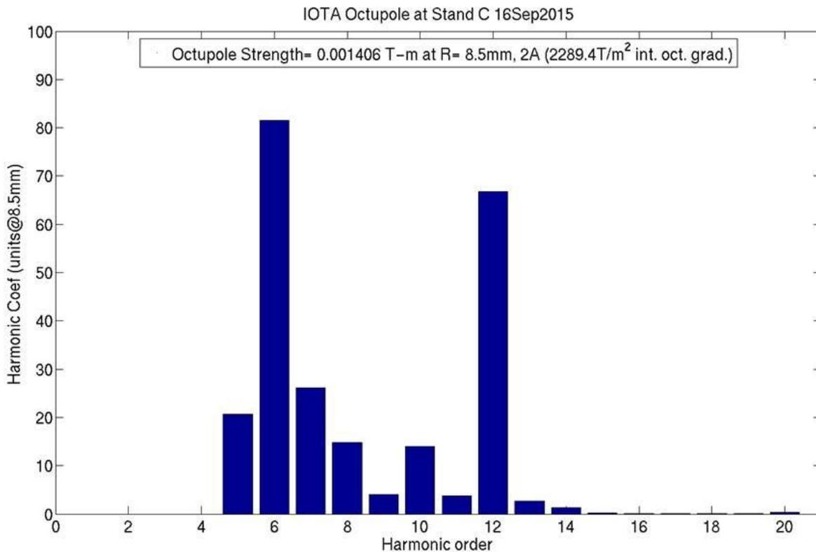
Figure 8 The harmonics of the octupole field at 8.5 mm from the magnetic center
