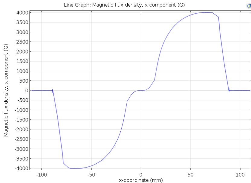
Figure 5 Comsol plot showing flux norm along x axis
