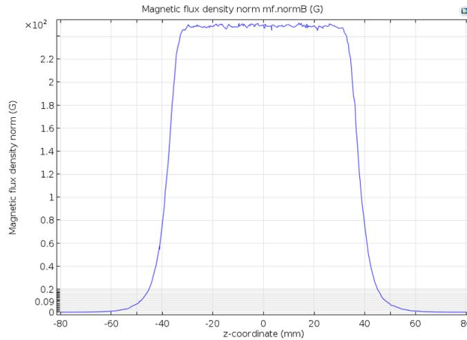
Figure 3 Comsol plot showing B magnitude along z-axis at 10 mm from the center
