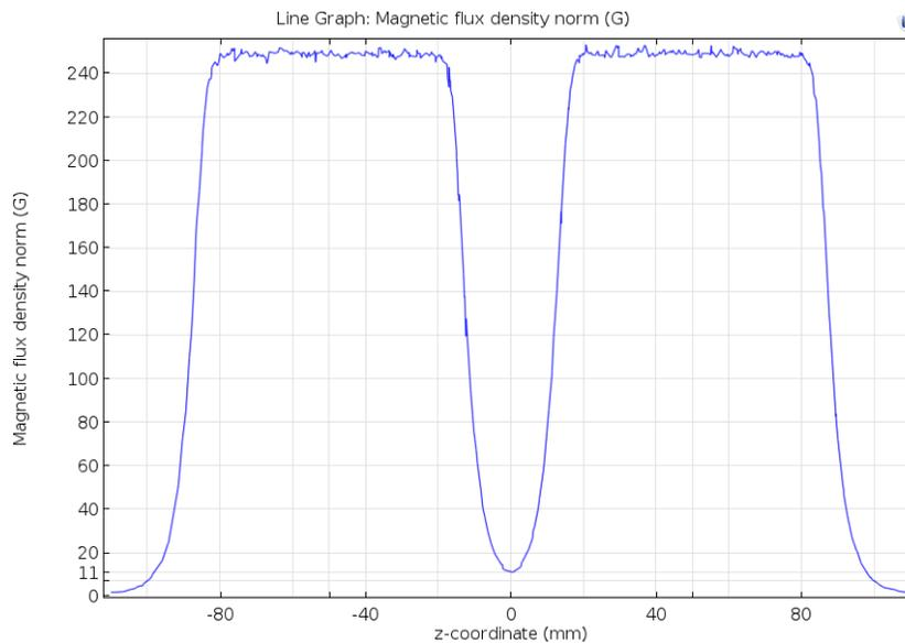
Figure 4 Comsol plot showing B magnitude along z-axis at 10 mm from the center for two magnets both powered at 2A
