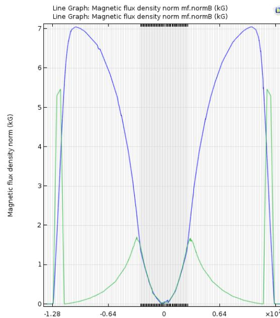
Figure 9 COMSOL plot showing the flux norm along the pole axis (blue line) and a perpendicular axis (green line)
