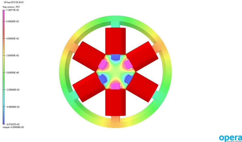
Figure 10 OPERA model showing magnetic potential
