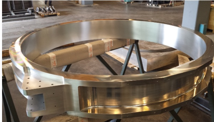
Figure 8.4: Prototype of the aluminum outer ring of the electromagnetic calorimeter at the INFN National Laboratory in Frascati.
