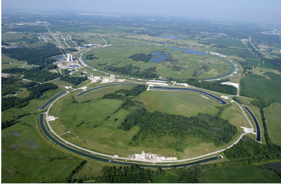
Figure 1.3: Aerial view of the Fermi National Accelerator Laboratory. The 3.2 km circumference Main Injector tunnel is visible in the foreground, the Tevatron tunnel is visible in the background. The Mu2e facility is located next to the High Rise. The Tevatron has been the most "powerful" particle accelerator for many years before the turning on of the Large Hadron Collider (LHC) at CERN in Geneva.
