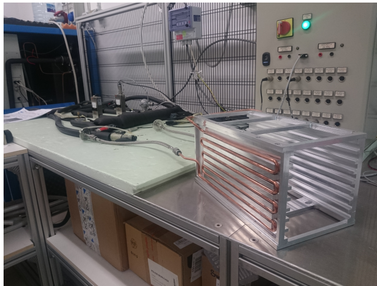
Figure 8.3: DAQ crate during hydraulic test.
