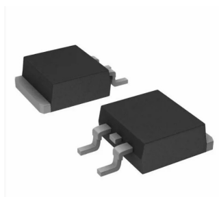
Figure 6.6: Power resistors used for the thermal test of the dummy waveform digitizer board.
