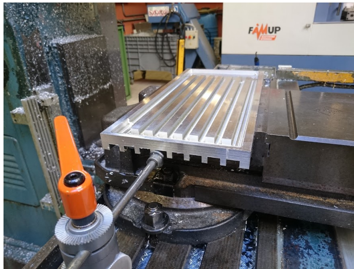
Figure 8.1: DAQ crate wall during the manufacturing process.
