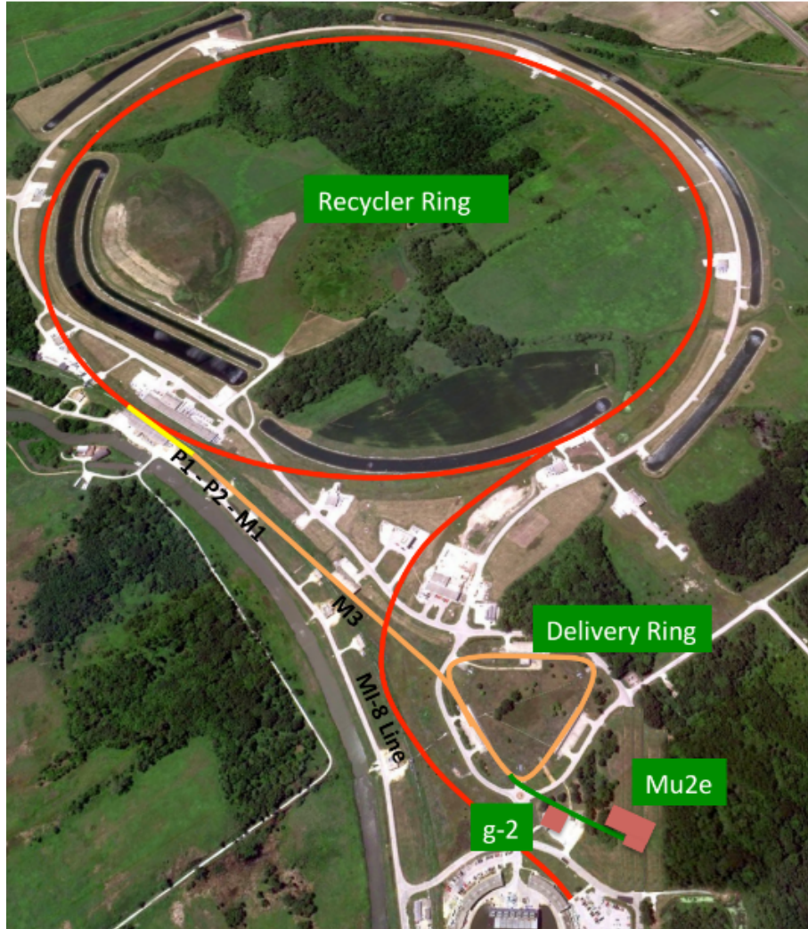
Figure 1.4: Layout of the Mu2e facility (lower right) relative to the accelerator complex that provides the proton beam to the detector. Protons are transported from the Booster through the MI-8 beamline to the Recycler Ring where they circulate while they are re-bunched by a 2.5 MHz RF system. The reformatted bunches are kicked into the P1 line and transported to the Delivery line where they are slow extracted to the Mu2e detector through a new external beamline. [12].
