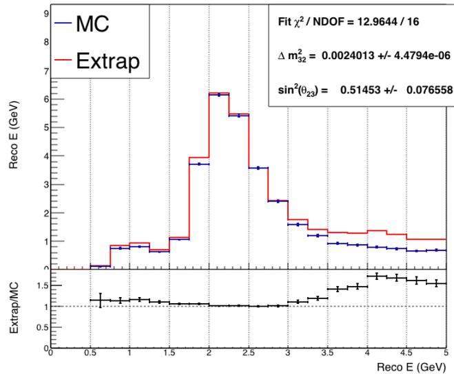
(b) Reconstructed energy spectrum in the Far Detector, without any systematics. The red line represents the result of the extrapolation, while the blue dots are the MC predictions.
