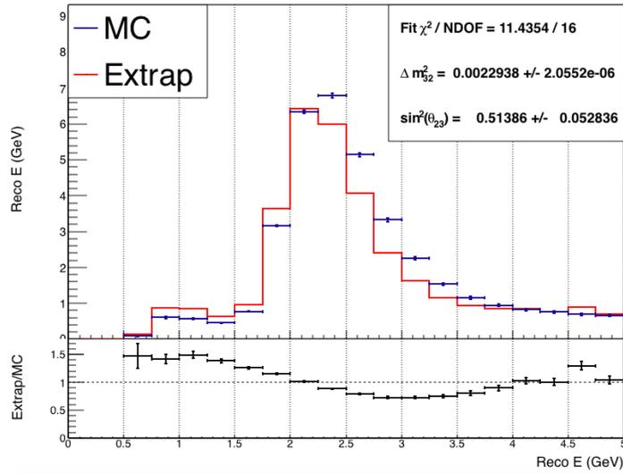
(b) Reconstructed energy spectrum in the FD after applying the Hadronic Absolute Shift High.
