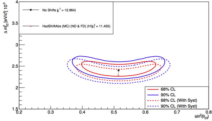
(a) Confidence level contours before (continuous lines) and after (dashed lines) having applied the Hadronic Absolute Shift High. The new best-fit point is still placed inside the confidence region.
