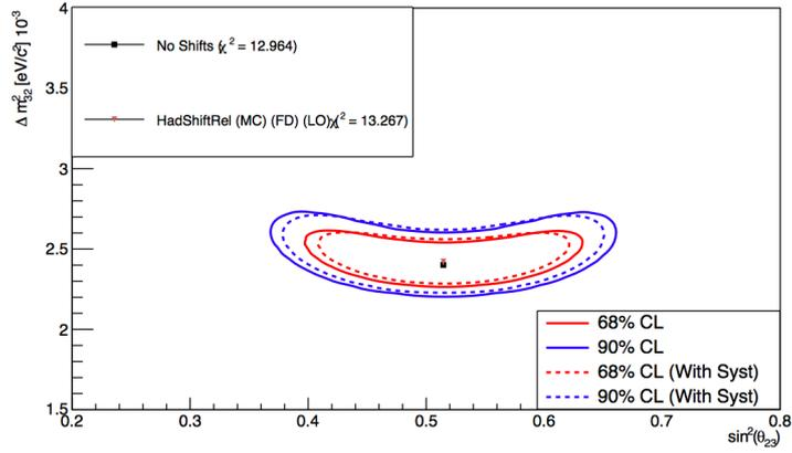
(a) Confidence level contours before (continuous lines) and after (dashed lines) applying the Hadronic Relative Shift Low.
