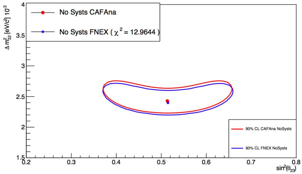
**Figure 7:** 90% Confidence intervals, gained with the CAFAna approach (red line) and the FNEX one (blue line). The direct comparison between them shows a tiny relative shift.
