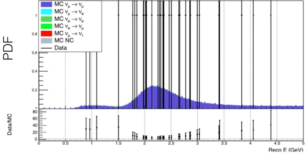
(a) Preliminary result for a simulated Probability Density Function (PDF), defined for use by a more general Unbinned Likelihood best fit. The black lines represent the collected data of the first  $\nu_\mu$  disappearance analysis, and the corresponding value of the PDF related to their energy.
