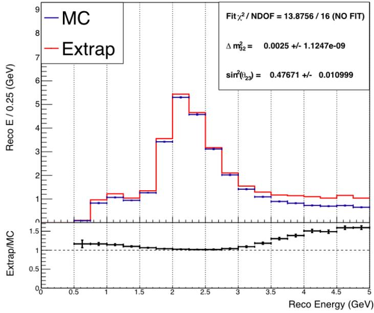
(a) *FD RecoE spectrum produced without any systematics and with the FNEX default method for the weights estimation. The contribution of each event to the recoE spectrum is weighted by its true energy.*
