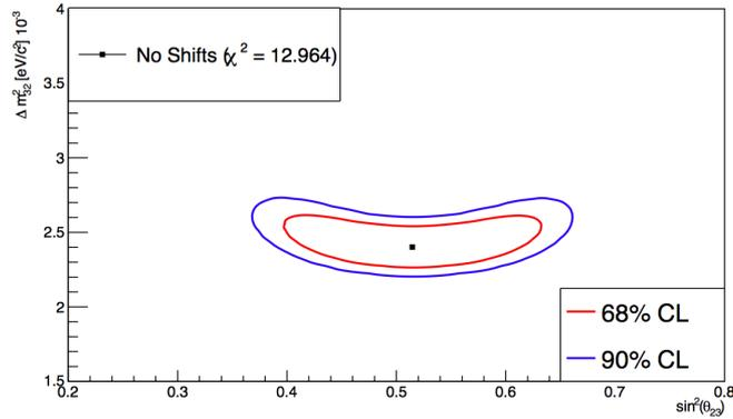
(a) Confidence intervals gained as output of a  $\nu_\mu \rightarrow \nu_\mu$  oscillation first analysis job in FNEX, without any systematic shift applied.
