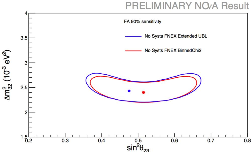
(b) Confidence level contours comparison without systematics, between the FNEX Binned  $\chi^2$  fit (red line) and the FNEX Unbinned Likelihood fit (blue line). The latter looks wider and the new best-fit point is shifted to a lower value of  $\sin^2 \theta_{23}$ .
