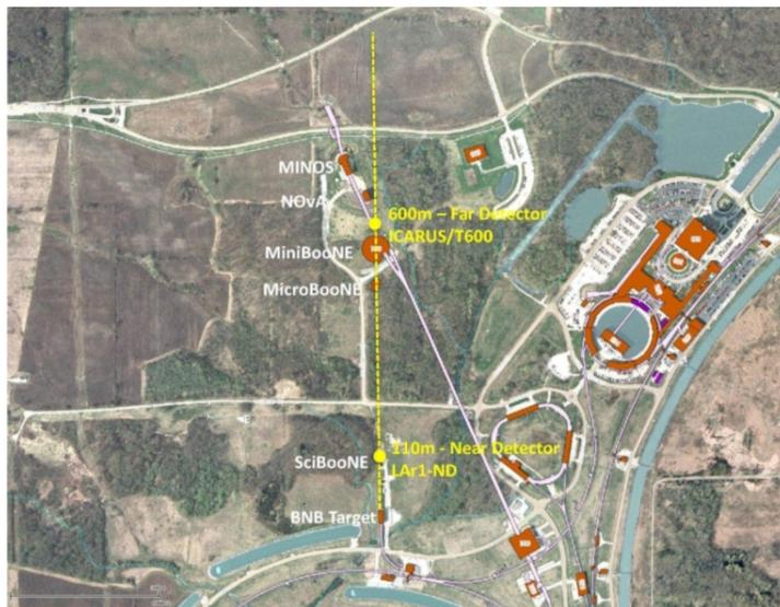
Figure 5: Map of the Fermilab neutrino beamline area showing the axis of the BNB (yellow dashed line) and approximate locations of the SBN detectors at 110 m, 470 m, and 600 m. The pink line indicates the axis of the NuMI neutrino beam for reference.
