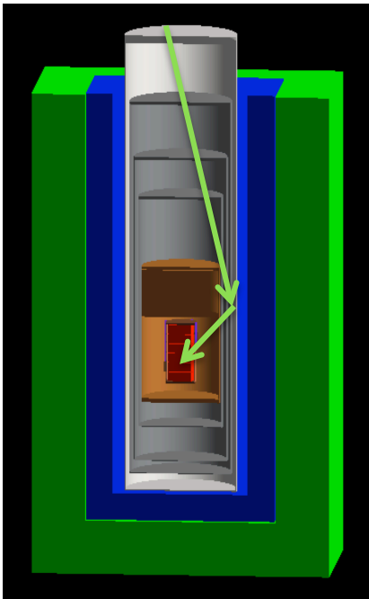
(a) Gamma rays possible path around the shielding.
