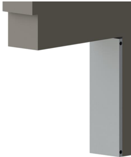
Figure 20 Cold plate installed on the stalactite's side
