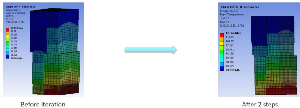
Figure 13 After two cycles, the maximum conceptual temperature in the blocks rises by 23°C
