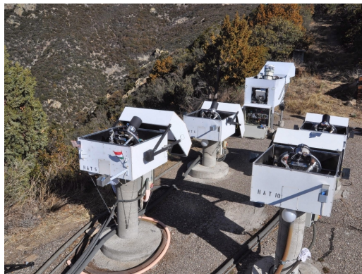
Figure: HATNet telescopes at FLWO, open for servicing during the day, and the HATNet telescope mount, camera, and lens. Photo credit: Gaspar Bakos.
