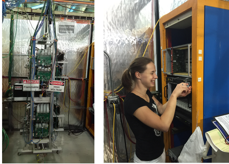
Fig.13: The cosmic ray telescope in FTBF and installation of devices for pLAPPDs running and readout.
