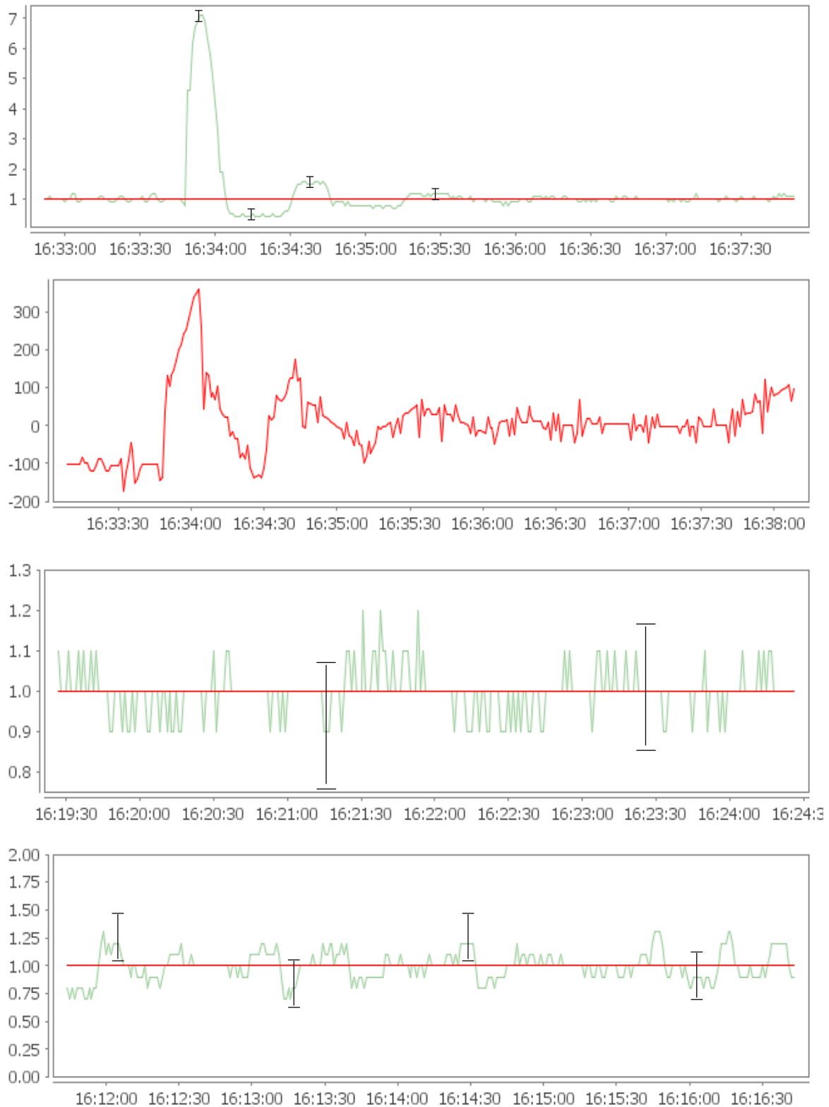
Fig. 15: Top to bottom four plots recorded during the tuning of the cavity. 1, 3 and 4 display the actual phase and the set point (phase in degrees vs. time [h min sec]); the uncertainty bar corresponds to \pm 0.2^\circ in all cases. 2 shows the output of the loop computation (number of steps vs. time).
