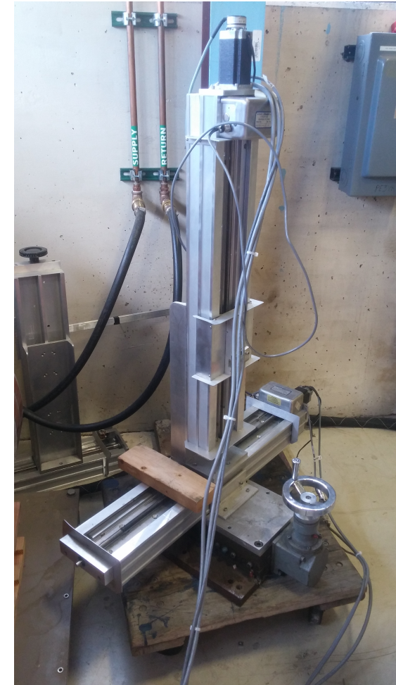
2 Axis motor used to map the magnet
