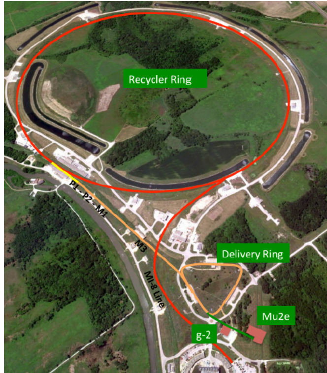
Fig. 1.4: Layout of the Mu2e facility (lower right) relative to the accelerator complex that provides the proton beam to the detector. Protons are transported from the Booster through the MI-8 beamline to the Recycler Ring where they circulate while they are re-bunched by a 2.5 MHz RF system. The reformatted bunches are kicked into the P1 line and transported to the Delivery Ring where they are slow extracted to the Mu2e detector through a new external beamline [5].
