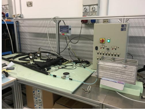
Fig. 5.3: Pressure loss test apparatus at INFN of Pisa. On the right the crate prototype connected to the two pressure gauges.
