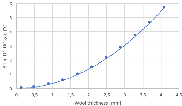
(b) Graph of the temperature drop caused by the copper wool gap filler.
