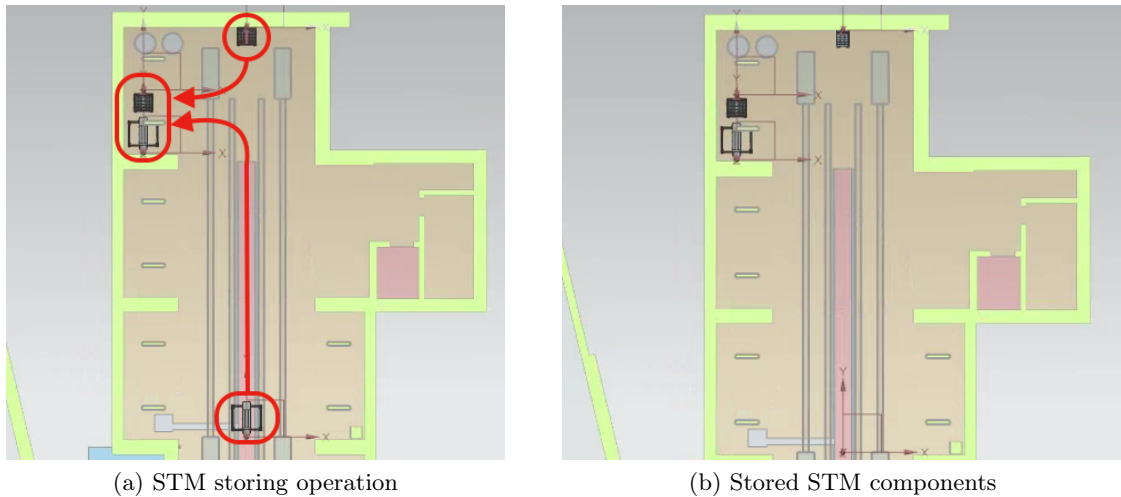
Figure 16: Storage of the STM components during maintenance
