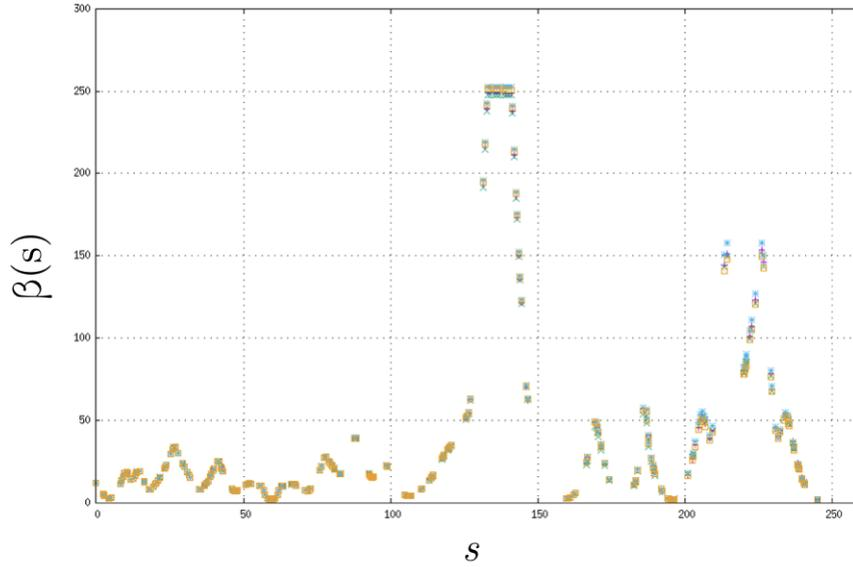
**Figure 12:** Modification of the  $\beta(s)$  function with quadrupole's field random errors. Each color represents a different run.
