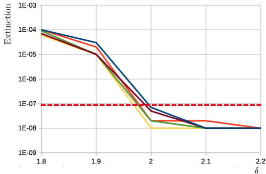
**Figure 13:** Extinction level as a function of  $\delta$  for quadrupole fields random errors. The different colors represent the five runs. The dotted line marks the level required.
