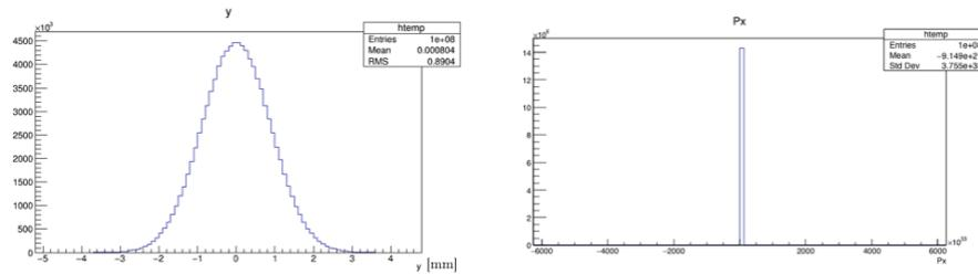
**Figure 9:** On the left: displacement distribution in the  $y$  direction. On the right: distribution of the  $x$  component of the momentum.
