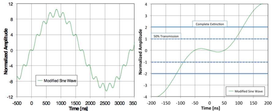
**Figure 6:** Final AC dipole waveform. On the left is the waveform over a complet cycle and on the right is the waveform over the transmission window.
