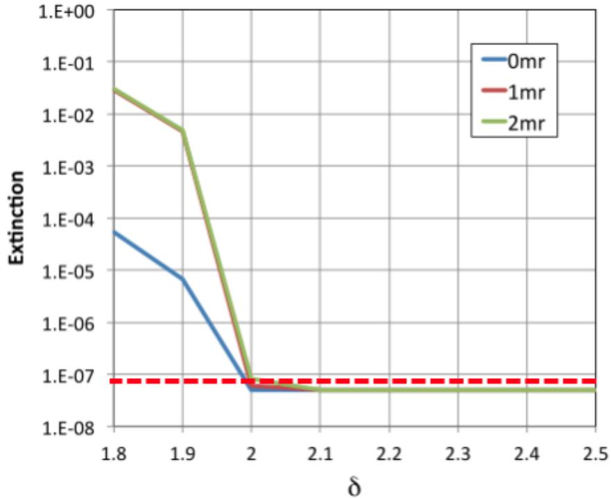
Figure 11: Extinction level as a function of the  $\delta$  and for  $\alpha = 0$  mr, 1 mr and 2 mr. The dotted line marks the level required.
