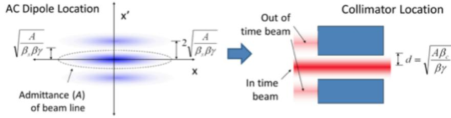
**Figure 5:** The blue clouds represent the beam in the phase space where the upper e lower halos are the out-of-time beam and the darker blue bunch is the in-time beam. On the right, a scheme of the downstream collimator where the red halos are the out-of-time beam having been deflected against the jaws.
