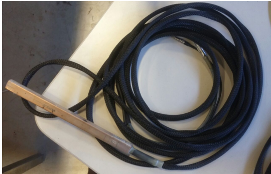
Figure 16: NMR Probe with cable.
