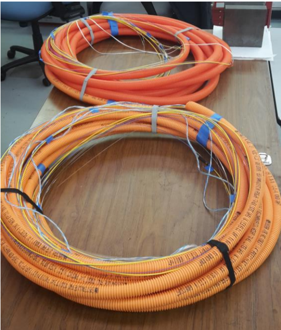
Laser and fibers for the local monitor inside the straw
