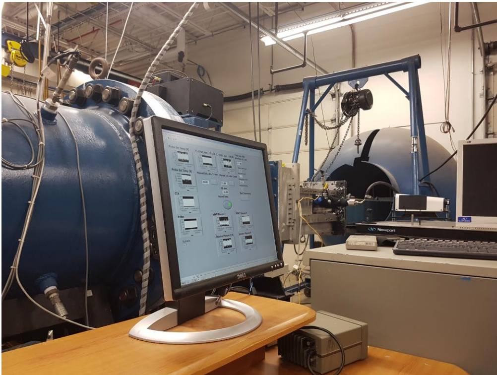
Figure 20: LabView program for the data acquisition and control of the Supersonic Wind Tunnel at UTA
