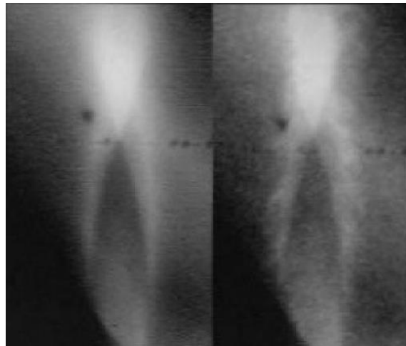
Figure 11: Ultraviolet Rayleigh images of an overexpanded supersonic nitrogen jet. The left image is time averaged and the right image is instantaneous. [6]
