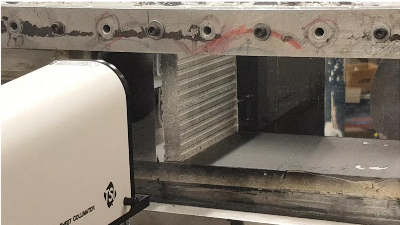
Figure 24: Alignment process for the FRS experiments; collimator and calibration plate
