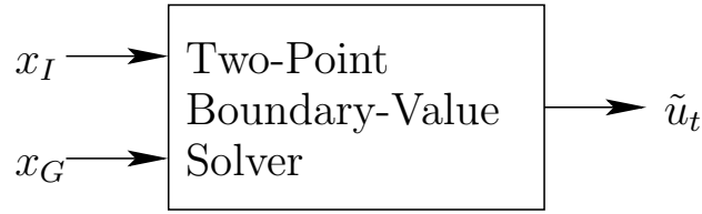
Figure 5.4: The BVP is treated as a black box that gives a control sequence as an output for any couple of start and end points.
