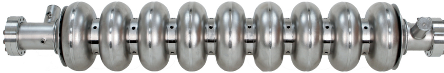
Figure 1: Nine cell 1.3 GHz Niobium Superconducting radio-frequency cavity.
