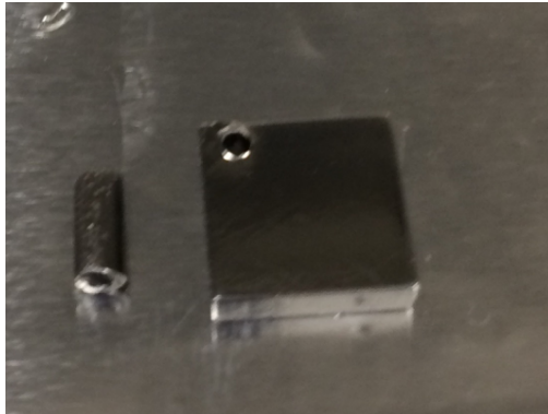
Figure 5: CaptionThe two kind of niobium samples treated, at left the cylinder for PPMS measurements and at right the 1x1 cm coupon for the other characterizations.
