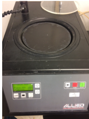
Figure 18: The polishing paper is stuck on the circular plate. The plate can spin and the sample is gently pressed on it by hand.
