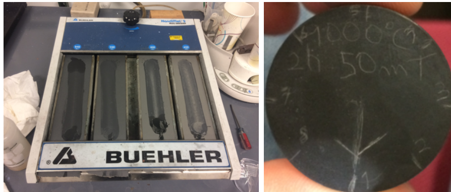
Figure 17: On the left there is the by-hand polishing machine, the grit of the paper is increasing from left to right. On the right there is a molded sample divided in section for the polishing.
