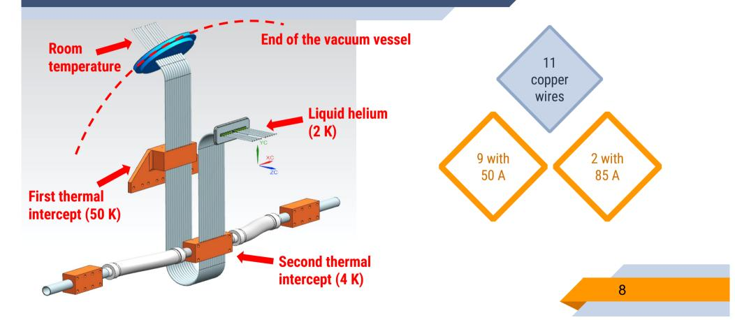
How can we be sure that the temperature of the wires reaches 2 K? How can we decrease the amount of heat flowing into liquid helium? How can we improve the system?
