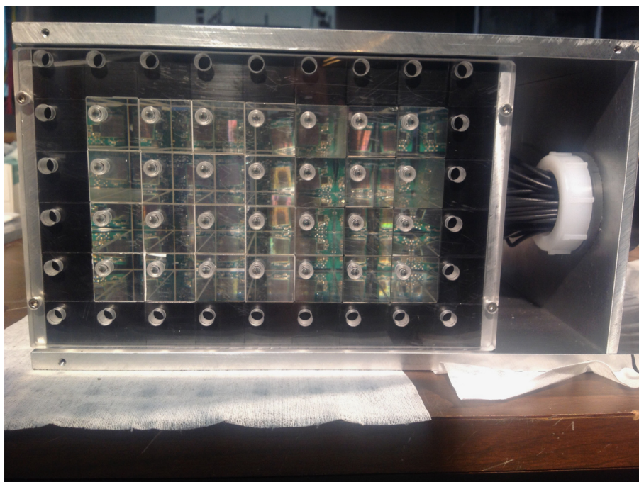
Figure 1.7: Calorimeter prototype tested at SLAC. Here it was used a smaller setup with 7x4 crystals.
