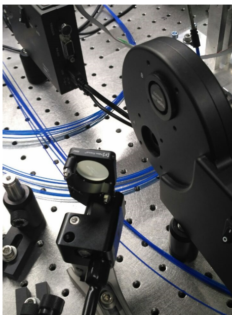
Figure 3.2: Motorized mount used to move the mirrors in and out from the light path. On the right, a motorized filter wheel.
