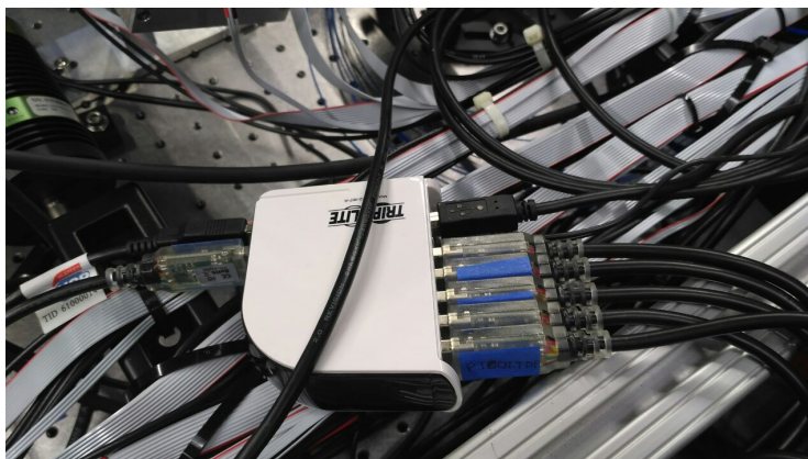
Figure 3.5: The six USB-to-TTL cables are plugged into the same USB hub.
