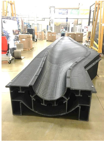
Figure 17: Wind turbine blade with additive manufacturing.
