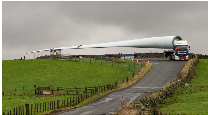
Figure 16: Wind turbine blade transportation.
