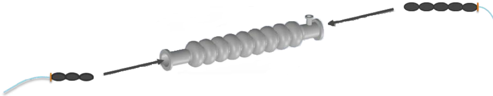
Figure 6: Deflated and folded balloons are placed inside the cells, apart the target cell, that in this case is the cell number 4.
