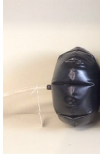
Figure 4: Rubberized nylon single cell balloon
