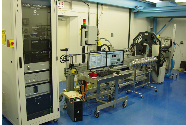
Figure 2: Automatic tuning machine (Courtesy: Fermilab)
