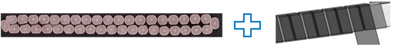
Figure 2.1: Strands and insulation
