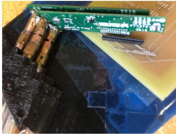
Figure 3.2: Mounted preamplifiers on the 3D mockup.
