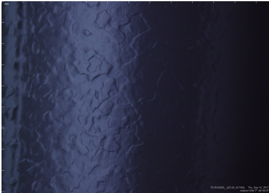
Figure 27: TE1AES024: Another region of the cavity (board 23, thermometer 19) showing pronounced steps at the grain boundaries.
